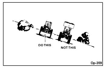
When transporting the load, keep bucket as low as possible, to avoid tipping, in case a wheel drops in a rut.
